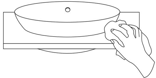
5. Let the assembled vanity sit for 24 hours to allow all the silicone sealant to fully dry. Once dry, proceed to the installation of your faucet and drain assemblies.
