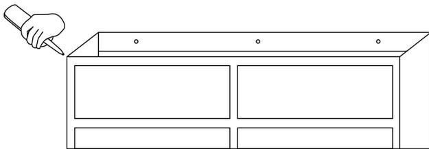
3. With assistance from another person, slowly and carefully set the top onto the vanity cabinet. Once positioned, press firmly into place. Wipe away any excess sealant using a damp cloth.
