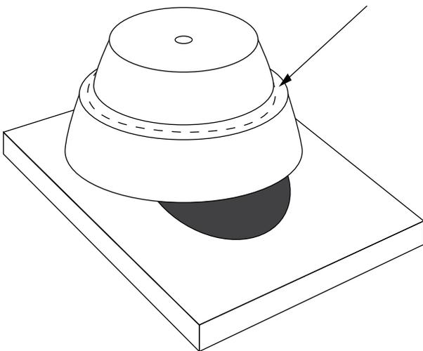
3. Turn the sink back over, placing it inside the sink's cutout and adjust the sink as necessary until centered. Once in position, press the sink firmly into place.
