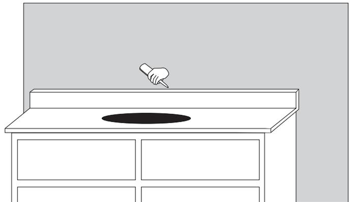
5. For stone tops, such as marble and granite, it is recommended that you apply a high-quality sealer to protect from staining and discoloration. Stone sealer should be reapplied once or twice per year, depending upon usage.
