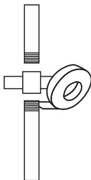
7. Complete the installation by installing the shower head onto the upper riser pipe.
