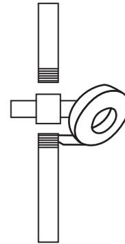
4. Complete the installation by installing the shower head onto the upper riser pipe.
