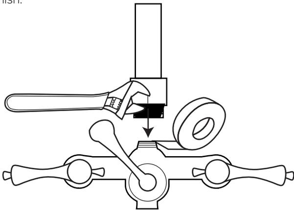
3. Insert the upper riser pipe through the mounting hole located on the shower curtain rod. Attach the upper riser pipe by threading it into the lower riser pipe. Apply a bit of thread sealant or plumber's tape to the threads before tightening.
