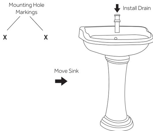
3. Drill pilot holes at the marked locations of the sink's mounting holes. If using anchors, insert the anchors into the drilled holes.
