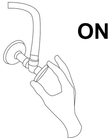
6. Turn the faucet on for approximately 60 seconds to check for any leaks. Ensure that both hot and cold water are functioning properly.
