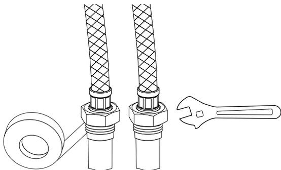
5. Once installation is complete, turn the main water supply back on from below the sink. Check for any leaks.
