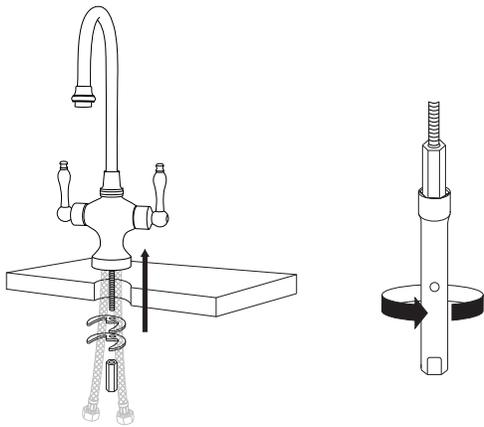
4. Attach the braided water lines to the main water supply. Ensure that the hot and cold lines are connected as marked. Apply plumber's tape or thread sealant to the threads before tightening. Hand tighten the connections, then finish tightening with an adjustable wrench. Be very careful not to overtighten.
