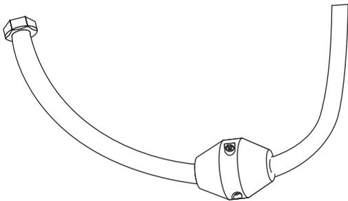
6. Attach your main water lines to the copper water supply posts on the faucet. Ensure that you are connecting the hot and cold in accordance with the labels on the supply posts. Apply a bit of thread sealant or plumber's tape to the threads before tightening.
