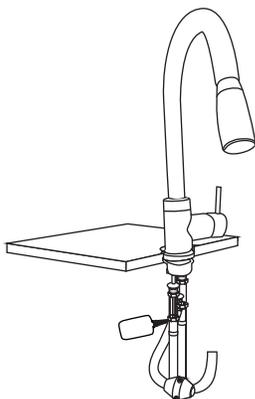
7. Once installation is complete, turn the main water supply back on from underneath your sink. Check for any leaks underneath.
