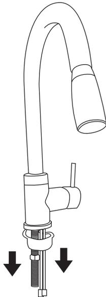
3. From beneath the sink, slide the brass spacer back onto the faucet body. Thread the locknut back onto the threaded shank until hand-tight to secure. Finish tightening using an adjustable wrench.
