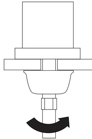
4. Attach the sprayer hose to its copper mounting post as shown. Insert the provided rubber O-ring into the lock nut before securing. Apply a bit of thread sealant or plumber's tape to the threads before tightening.
