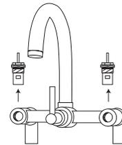
5. Place a small cup or other plastic container upside down over the cartridge cavity. Place a towel behind the faucet to prevent water from spraying out.
