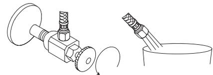
8. Close the shut-off valve or main supply, then reattach the water lines to the faucet.
