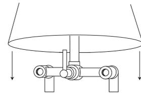
6. Holding the cup in place, turn on the hot water valve and let run for 3-5 seconds. Holding the cup in place, do the same for the cold water. This will dislodge any debris in the water line.
