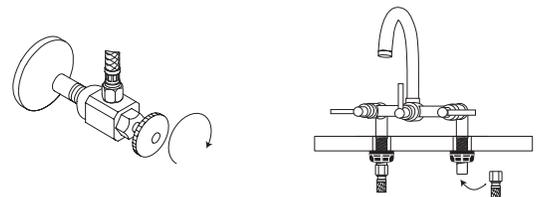
9. Reopen the valves to restore water to the faucet and check for leaks.
