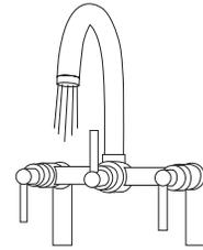
6. With a wrench, remove water lines underneath the faucet, placing the ends in a bucket.
