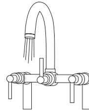
3. Remove the faucet handles by unscrewing the screw or set screw (depending on the style of your faucet).
