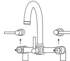
4. Loosen the locknuts and remove the cartridge(s), noting their positions (if reassembled in the wrong position, their handle action will be reversed).
