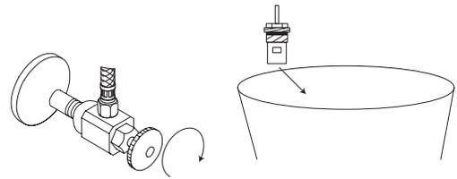
8. Reinsert the cartridge(s) in the correct position, then reassemble the trim and handle. Turn on the faucet to test water flow and check for leaks.
