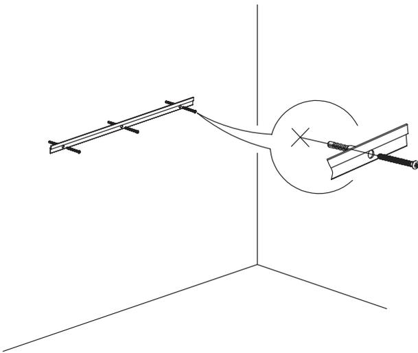
3. Attach the medicine cabinet to the mounting bar as shown, open the cabinet door, and make a mark on the wall with a pencil through the backplane hole (A).
