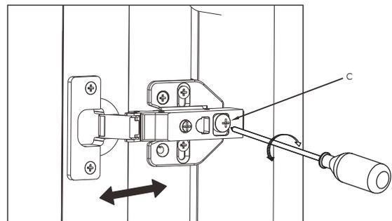
Rotate Clockwise: Distance between door and cabinet reduces.
