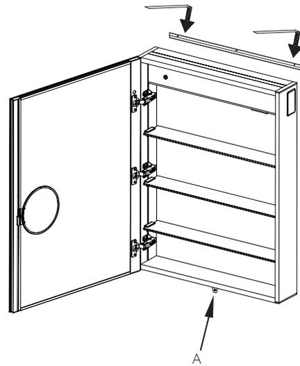
4. Remove the medicine cabinet, drill the mounting hole in the wall in the marked position, and place the wall anchors.
