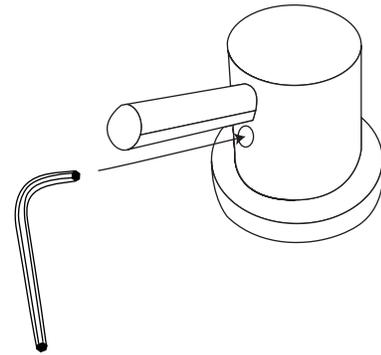
8. Repeat steps 4-7 to install the 'hot' valve stem into the left-side faucet hole.
