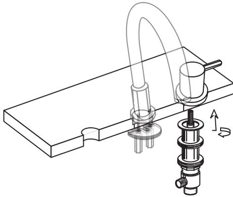
6. From beneath the counter top, tighten the lower lock nut until hand-tight. Finish tightening using a basin wrench.
