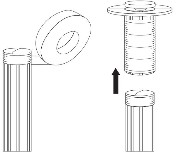
3. Slide the flat rubber gasket up the tailpiece until it meets the lip of the pop-up drain flange.
