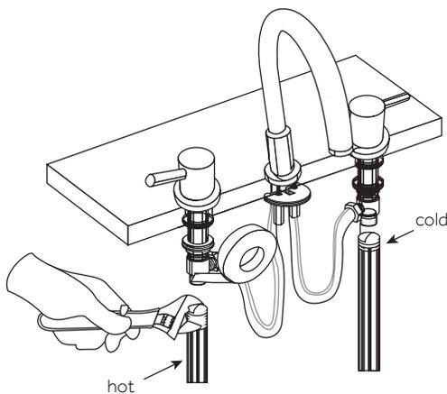
11. Once installation is complete, turn the main water supply back on from below your sink. Check for any leaks underneath.
