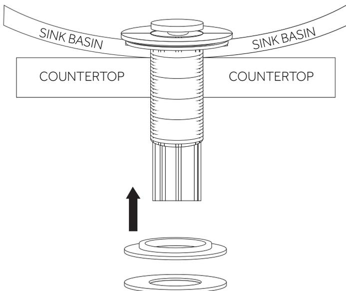
6. Thread the lock nut onto the drain flange. Hand tighten until secure, then finish tightening with an adjustable wrench once the drain is properly aligned.
