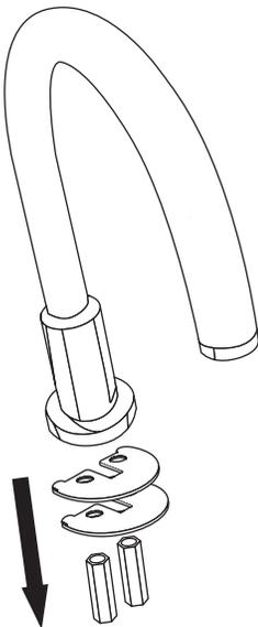
3. Set the spout into the center mounting hole. From beneath the countertop, slide the rubber gasket followed by the metal washer back onto the threaded mounting post. Hand tighten the lock nut, then finish tightening using an adjustable wrench.
