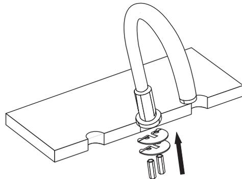
4. The faucet's valve stems are labeled – 'H' for hot and 'C' for cold. Remove the handle from the cold valve stem by loosening its set screw with the provided hex wrench. Remove the handle base, upper metal washer, upper rubber gasket, and upper lock nut from the valve stem as well.
