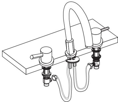
10. Attach the main water lines to the proper inlet on the bottom of each valve stem. Apply thread sealant or plumber's tape to each threaded connection. Ensure that you are connecting the hot and cold lines appropriately. Use an adjustable wrench to tighten, but be careful not to overtighten.
