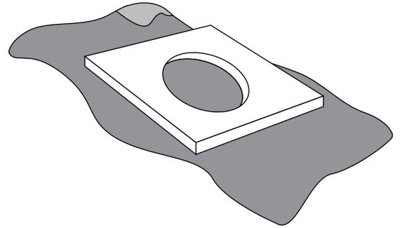
2. Position the sink over its cutout on the countertop. Make sure the sink is centered with the faucet hole and is evenly spaced between the bolt holes.
