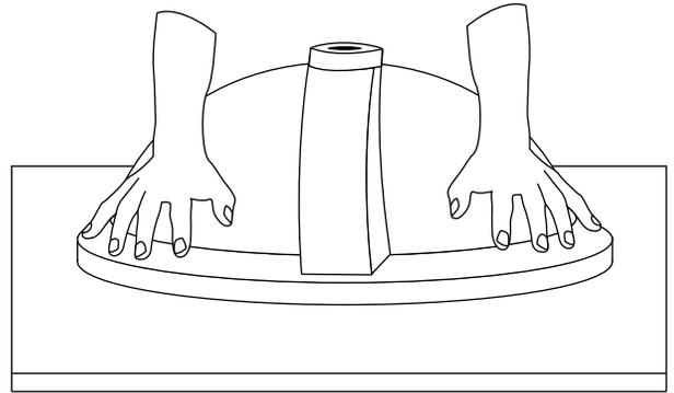
6. At each of the bolt holes in the countertop, attach sink clips by placing the long end of the bracket flat against the sink lip. Screw the wing bolts through the brackets and bolt holes and tighten.
