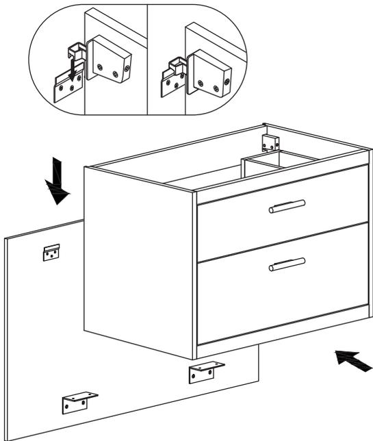
4. Adjust the mounting attachment as required. Lower screw adjusts vertical position. Upper screw adjusts depth.
