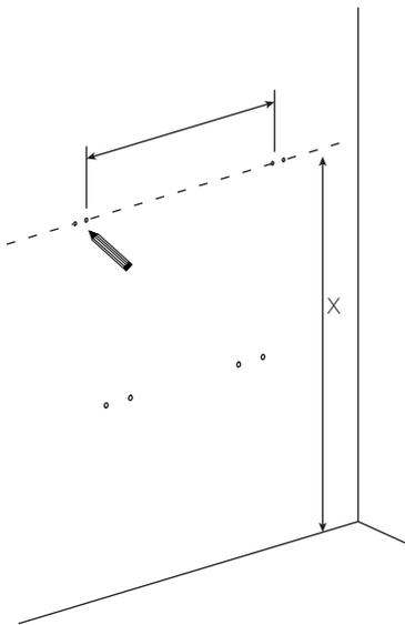
2. Drill pilot holes at marked mounting points. Insert wall anchors into the mounting holes for reinforcement. Align mounting brackets with pilot holes and secure with provided hardware.
