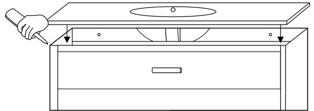
2. With assistance from another person, slowly and carefully set the countertop onto the vanity cabinet. Once positioned, press firmly into place. Wipe away any excess sealant using a damp cloth.
