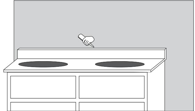
4. Allow the silicone sealant to dry. It will take up to 24 hours to dry completely.
