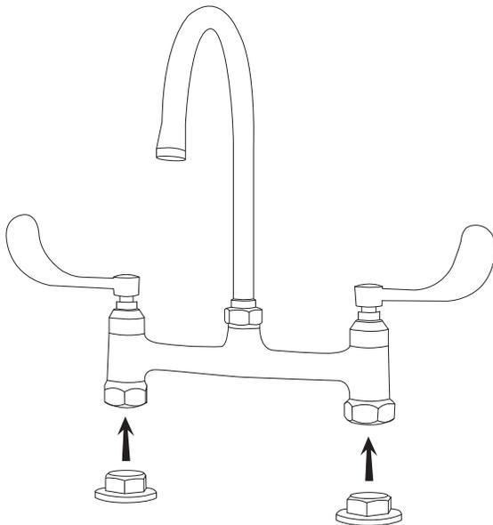
3. From below, slide the metal washers onto the threaded shanks. Thread the locknuts onto the shanks until hand-tight, then finish tightening using an adjustable wrench.
