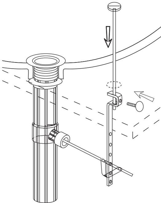
9. Make any final adjustments to the positioning of the link and drain lever as needed. Adjust until the drain fully opens and closes.
