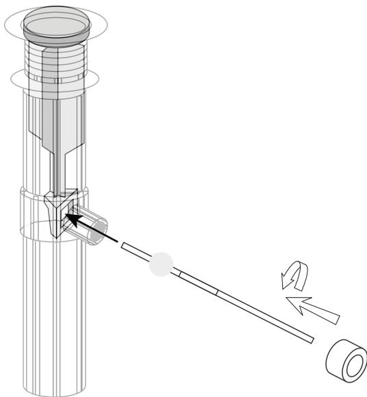
5. Position the drain so that the lever is facing the back of the fixture, in line with the faucet's lift rod. While holding in place, hand tighten the lock nut until secure then finish tightening with a basin wrench. Be careful not to overtighten, which can crack a fragile sink.
