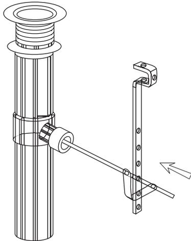
8. Attach the lift rod to the top of the link and secure it by tightening the thumb screw.
