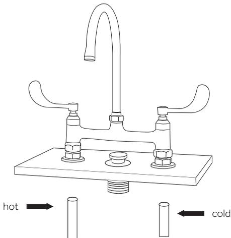
6. Once installation is complete, turn the main water supply back on from underneath your sink. Check for any leaks underneath.
