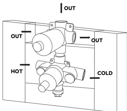
3. Route, assemble, and connect all in-wall piping as desired to and from the shower valve. Make all connections appropriately depending upon the type of pipe that is being used. For copper pipe, soldering will be required and should be completed by a licensed plumber. Apply plumber's tape to any threaded connections if applicable. Install any wood blocking that is necessary to support the piping and valve.
